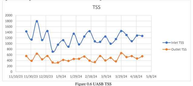
Figure 3.13 also shows the variation of TSS in UASB effluent ranging from 328 mg/L to 660 mg/L. The average TSS concentration in the UASB effluent was found to be 471 mg/L. An average TSS value of 471 mg/L indicates that the UASB reactor has significantly reduced the amount of suspended solids in the wastewater.
