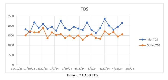
Figure 4.14 also represents the TDS in UASB effluent. The TSS range from 1280 mg/L to 1890 mg/L. The average TDS in UASB effluent were found to be 1535 mg/L.
