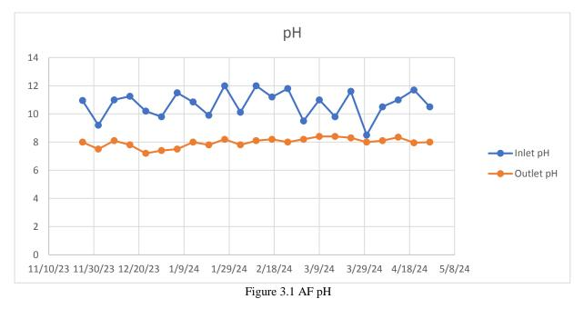
The pH of anaerobic filter effluent ranges from 7.2 - 8.4 which is within the optimal range. The average outlet pH is 7.96.
