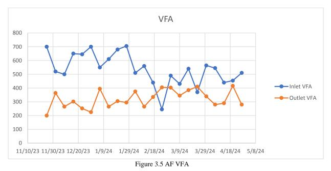
Figure 3.5 also shows the variation of VFA's in anaerobic filter effluent ranging between 200 mg/L and 416 mg/L. The average VFA concentration was found to be 321 mg/L.
