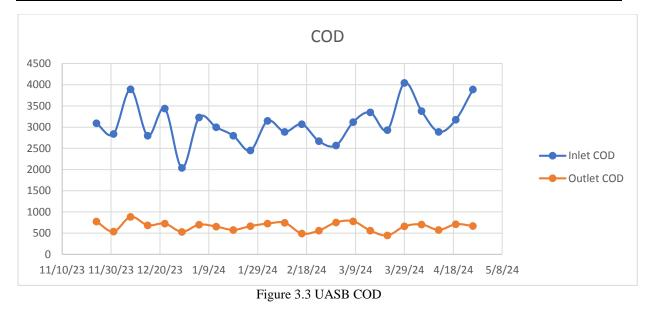
Figure 3.10 also shows variation in effluent COD. The effluent COD varied from 445-884 mg/L. The average COD concentration was found to be 657 mg/L.
