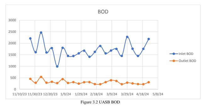
Figure 3.9 also shows the variation in BOD of the effluent ranging from 220 mg/L to 536 mg/L. The average effluent BOD for the entire period of the research was found to be 306.3 mg/L.
