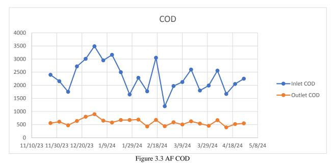
The effluent COD varied from 396-896 mg/L. The average COD concentration of the anaerobic filter effluent was found to be 593 mg/L. The COD removal was found to be 74%.
