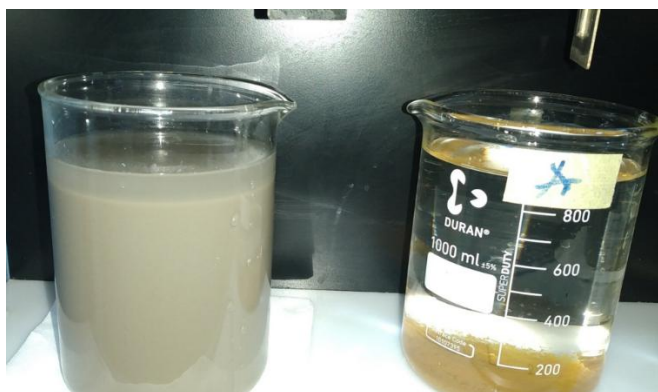
Figure 3.2; Picture showing Decolourization of the tailing and wastewater after coagulation experiment.
