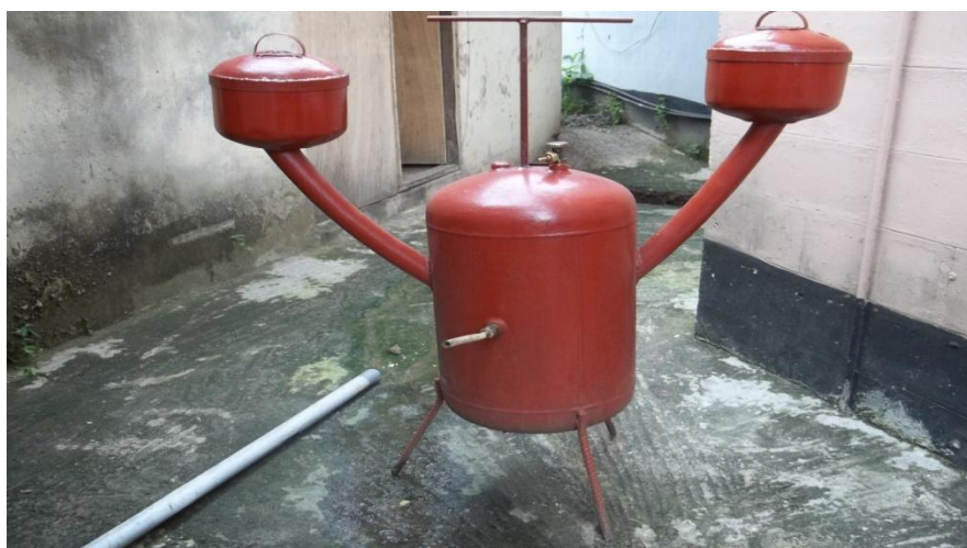
Plate 1: Showing photograph of constructed bioreactor
