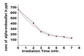
Fig.13 Degradation Profile of Alpha endosulfan under gamma irradiationn
