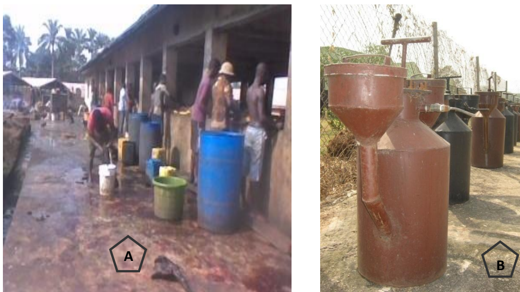
Fig. 3: (A) Cow dung washed into drainage at Nsukka abattoir; (B) Fifty kilogramme capacity prototype of Chinese fixed dome bioreactor located at the NCERD used for this study.
