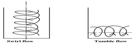
Fig 1 Swirl and Tumble flow in a cylinder.
