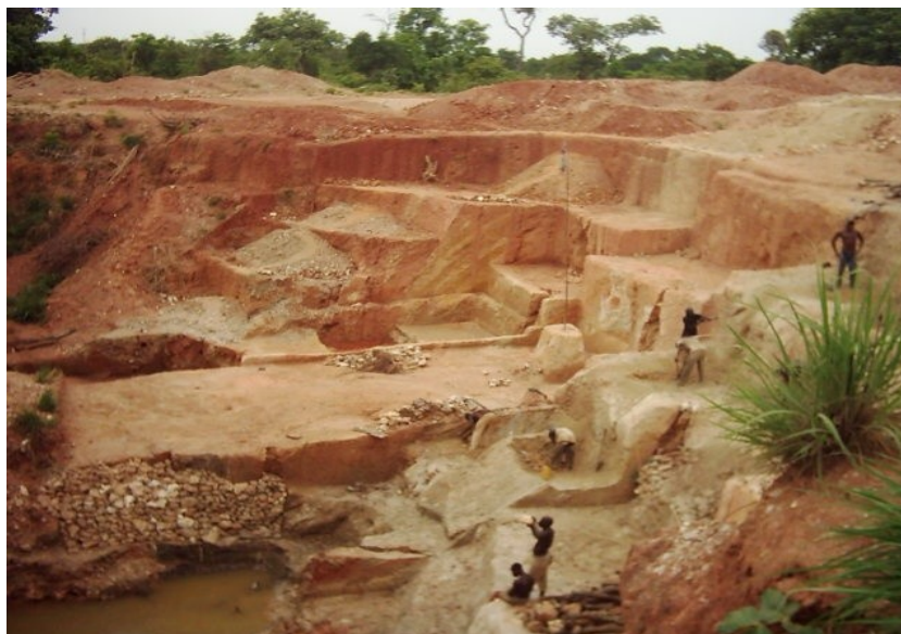
Fig. 1 Stepwise and relay system of moving debris at the mining site.
