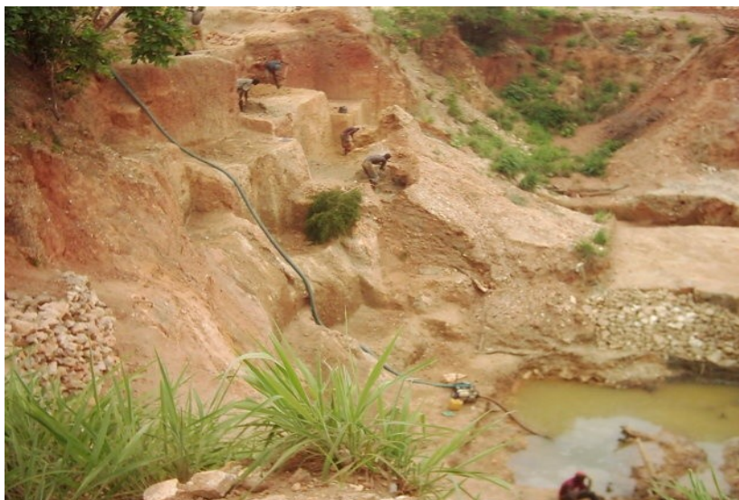
Fig. 3 Pumping machine draining water out of the mining pit .
