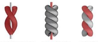
a. Metal-wrapped Yam b. Metal-filled Yam c. Metal Yar Figure 5: Structure of conductive yarns. Conductive material is shown in red<sup>[9]</sup>.
