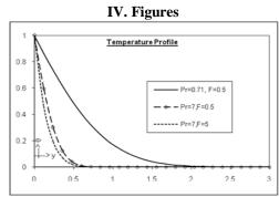
Figure-1 Temperature Profile showing the effect of Pr and F
