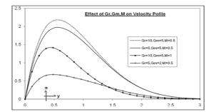
Figure-4 Velocity Profile showing the effect of Gr, Gm and M
