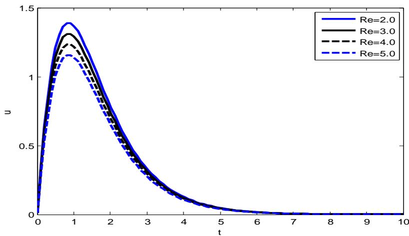
**Fig 8.** The velocity field  $u$  is depicted against  $t$  for different values of the Reynolds number  $Re$ .
