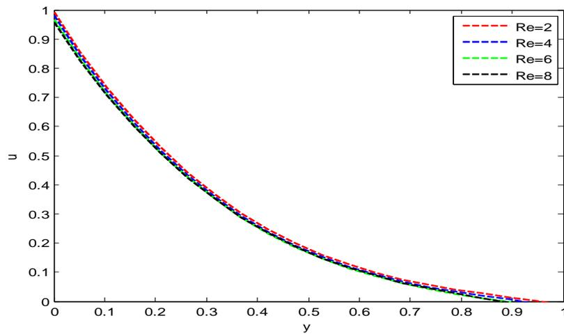
**Fig 7.** The velocity field  $u$  is depicted against  $y$  for different values of the Reynolds number  $Re$ .
