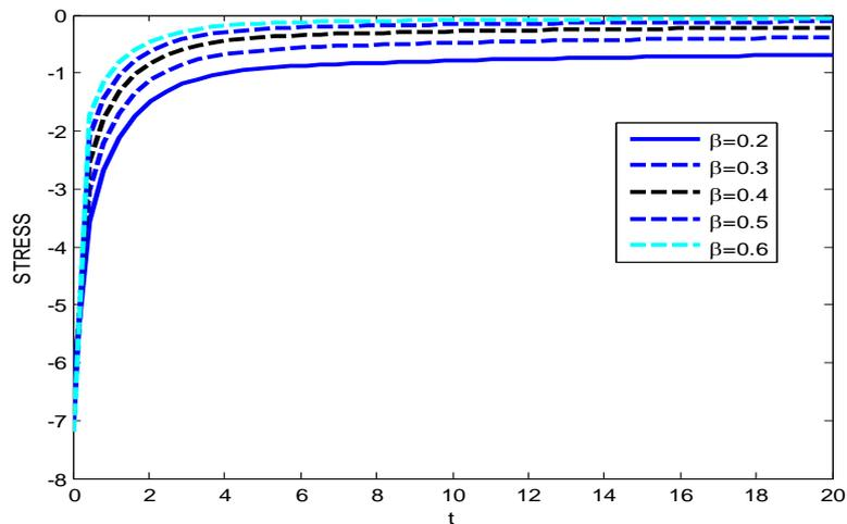
Fig 9. The stress field is depicted against time  $t$  for different values of the parameter  $\beta$ .  $\eta = 1.0$ ,  $\sigma = 1.0$ ,  $Re = 2.0$
