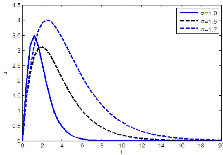
Fig 4. The velocity field  $u$  is depicted against time for different value of  $\sigma$ .  $\eta = 1$ ,  $\beta = 0.2$ ,  $y = 0.3$ ,  $Re = 2.0$
