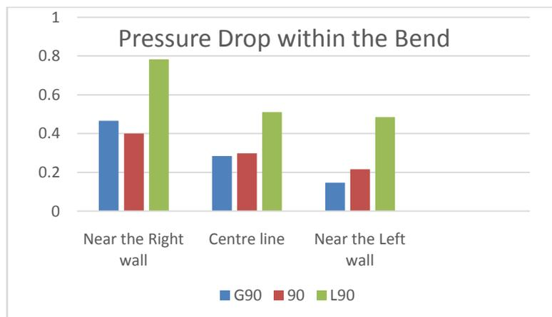
Figure.10: Pressure drop comparison along the bend among the three cases.
