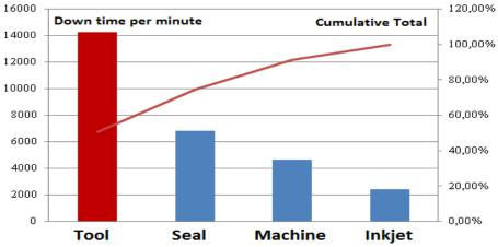
Figure 4: Pareto diagram of the machine sub-assembly
