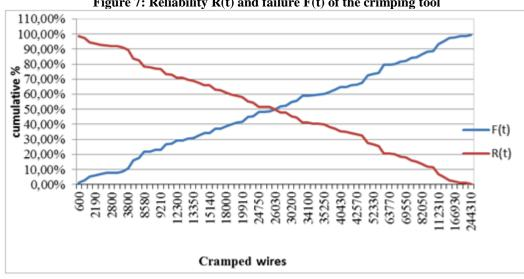
Figure 7: Reliability R(t) and failure F(t) of the crimping tool
