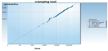
Figure 6: Visualization of TBF using Weilbul diagram
