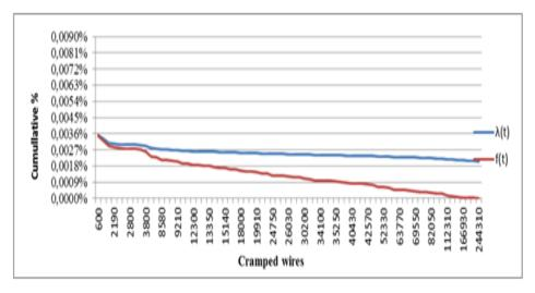
Figure 7: Failure rate of the cramping tool.
