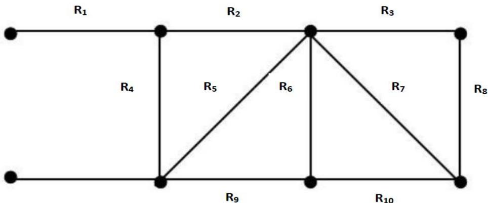
An undirected model representation of the circuit network with its edges is weight corresponding to the resistor value of each branch.
