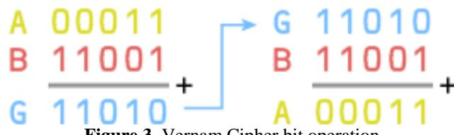
**Figure 3.** Vernam Cipher bit operation
