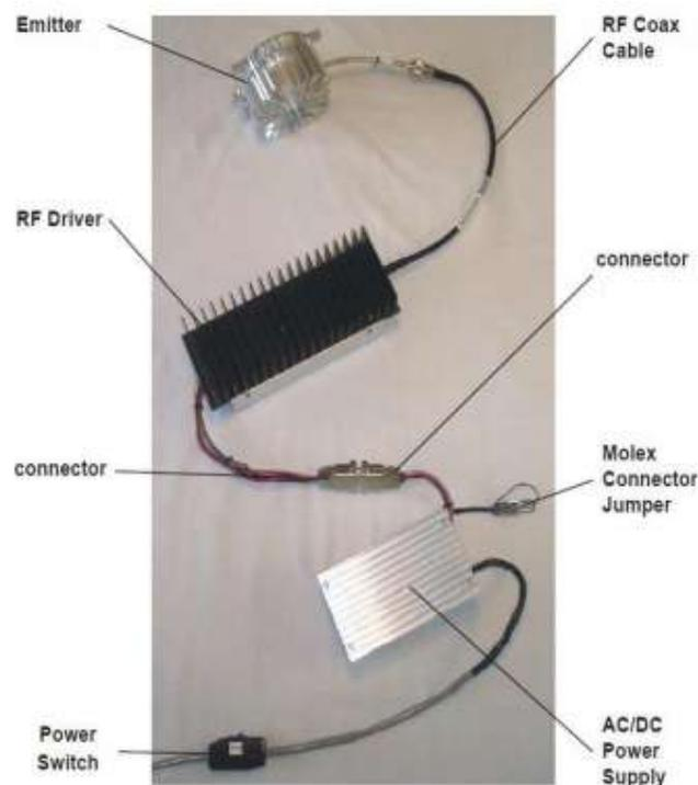
**Fig.17**Implementation diagram for Li-Fi
