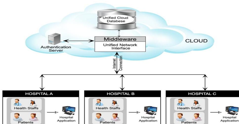
Figure 3: The Architecture of the PC-CBEHR System
