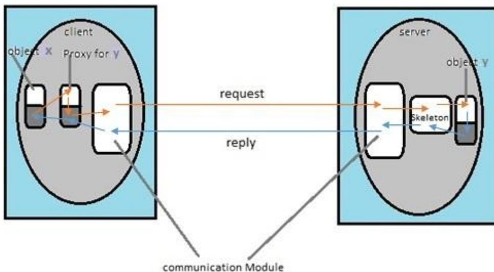
Figure 1. Request-reply view of Java RMI Architecture
