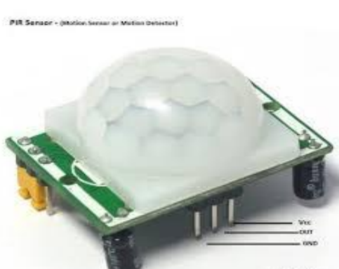
Fig. (e):PIR Sensor
