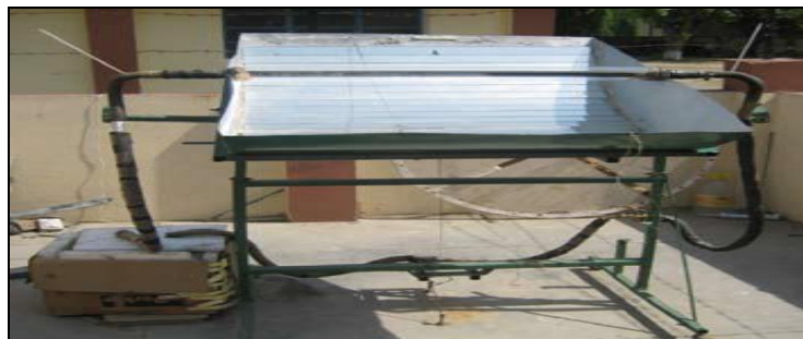
Fig. 1 Parabolic solar collector
