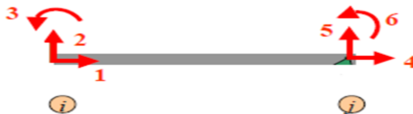
Fig. 7: Degree of Freedom of a plane frame element
