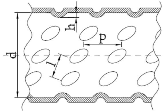
Fig 6. Dimple Spacing
