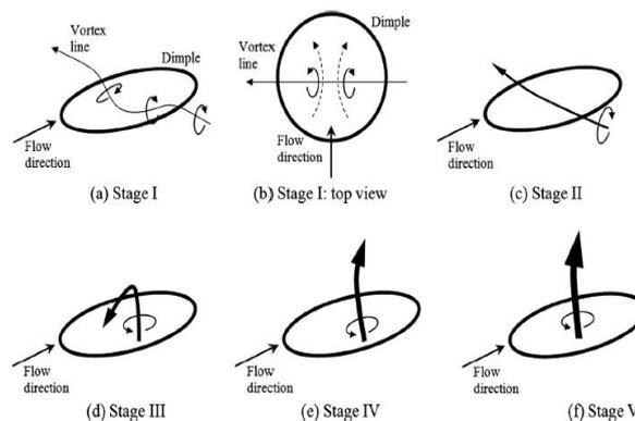
Fig 2. Flow in Dimpled Section
