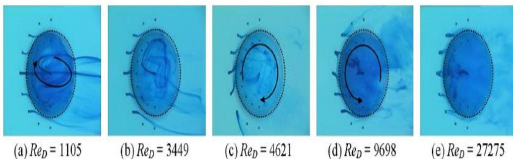
Fig 5. Dye Jet Showing Flow In Dimpled Section
