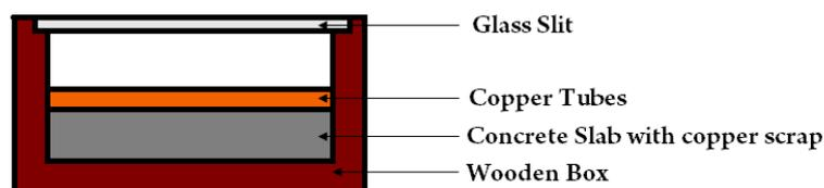
Fig.1 Schematic Diagram of Apparatus
