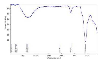
Fig 1: Fourier transform infrared spectra of spectra of pure silica produced from RHA
