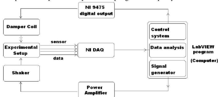
Fig 3 Structure of DAQ experiment
