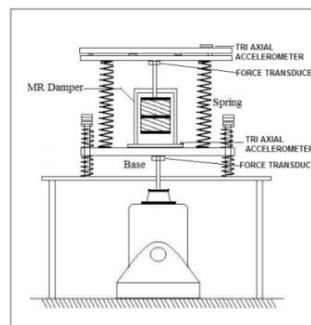
Fig 2 Schematic of Spring mass damper system
