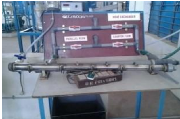
Figure 3. Experimental setup for Pipe Heat Exchanger with circular fins.
