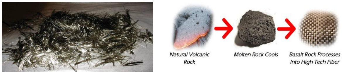
Fig 3: Basalt Conversion Process
