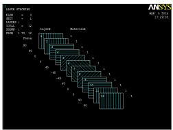
Fig 2: Symmetrical stacking sequence for [90<sub>2</sub>/0<sub>2</sub>/45/-45]<sub>s</sub>.
