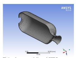
Fig 1: Finite element modeling of GFRP pressure vessel
