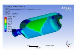
Fig5: Maximum shear Stress distribution for GFRP pressure vessel
