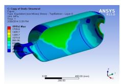
Fig 3: Equivalent Stress distribution for GFRP pressure vessel
