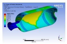
Fig 4: Maximum principal Stress distribution for GFRP pressure vessel
