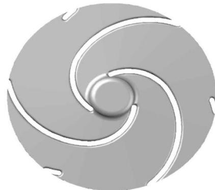
**Fig. 7 Model of modified impeller A**
