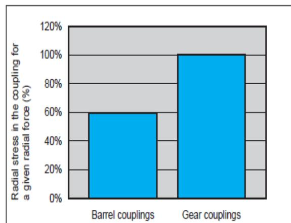
Fig. 3 Bending stress comparison of Barrel coupling and gear coupling
