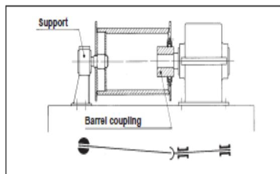
Fig. 1 mounting with barrel coupling
