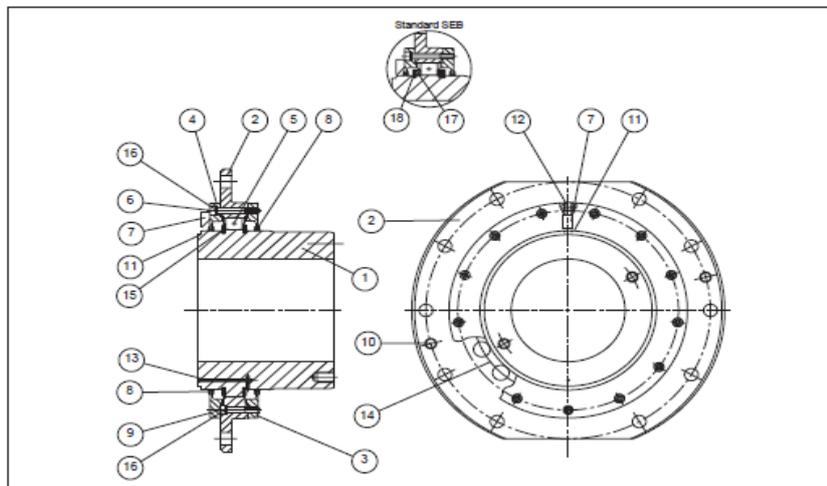
Fig.2 Components of barrel coupling
