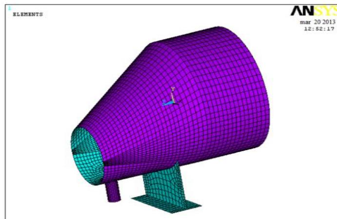
Fig.4: F.E.A. mesh model for design case
