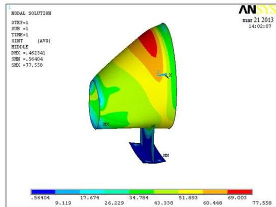
Fig.7 Cone with saddle middle layer stress intensity plot at design condition
