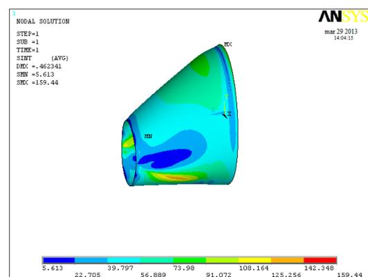
Fig.11 Cone without saddle bottom layer stress intensity plot at design condition
