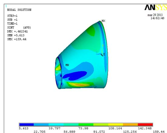
Fig. 9: Cone without saddle top layer stress intensity plot at design condition
