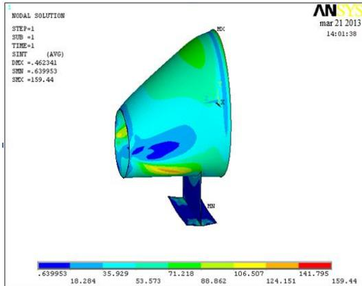
Fig.6 Cone with saddle top layer stress intensity plot at design condition
