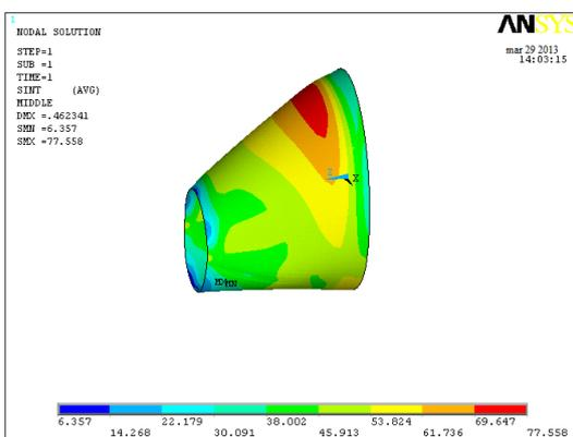
Fig.10 Cone without saddle middle layer stress intensity plot at design condition
