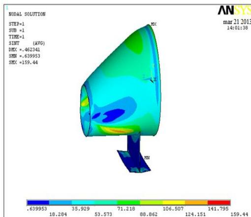
Fig. 8: Cone with saddle bottom layer stress intensity plot at design condition
