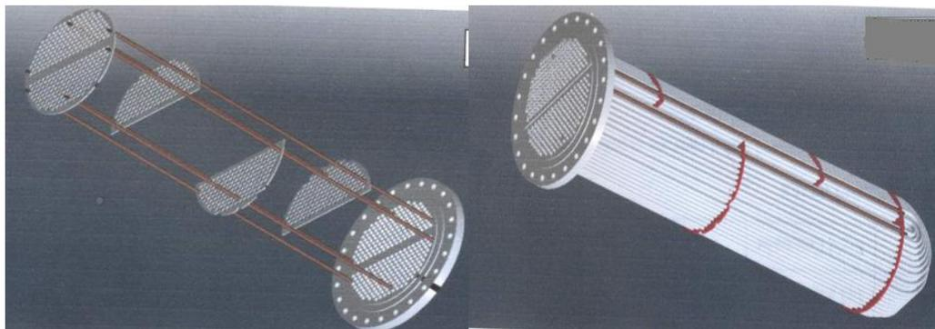
Fig.1 Tube sheet and baffle assembly
