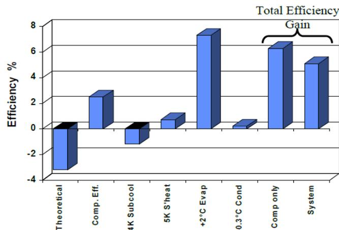
Fig. 2 Percentage efficiency effects for R410a, reference R22.
