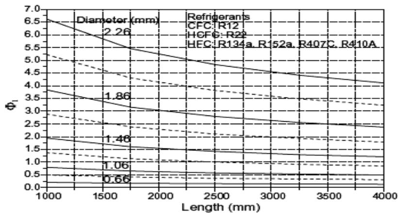
Fig. 8 Correction factor for capillary tube geometry.
