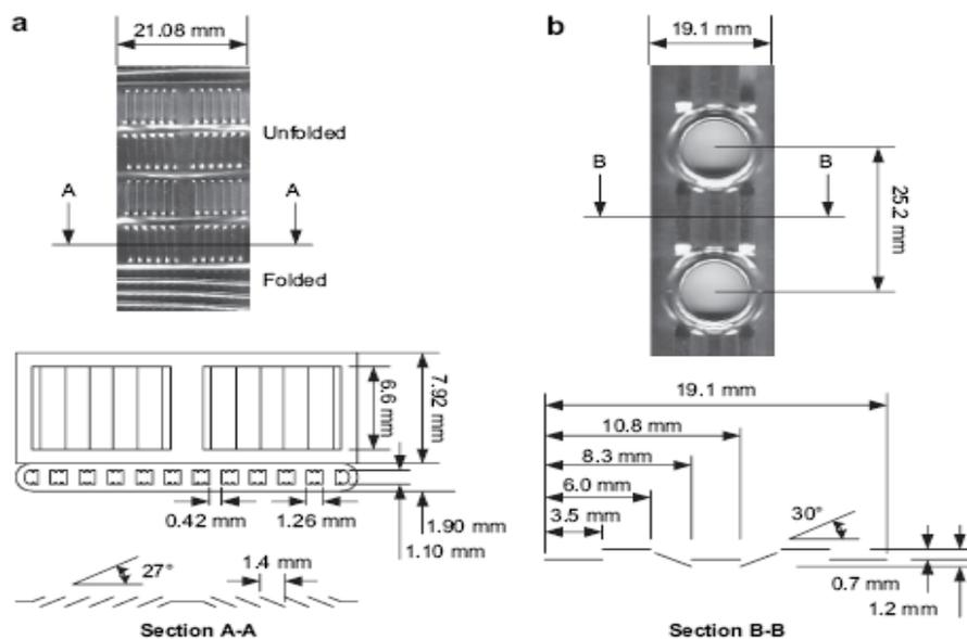
Fig. 5 (a) Louvered folded fins and micro-channel dimensions in the micro-channel condenser and (b) offset-strip plate fins in the round-tube condenser.
