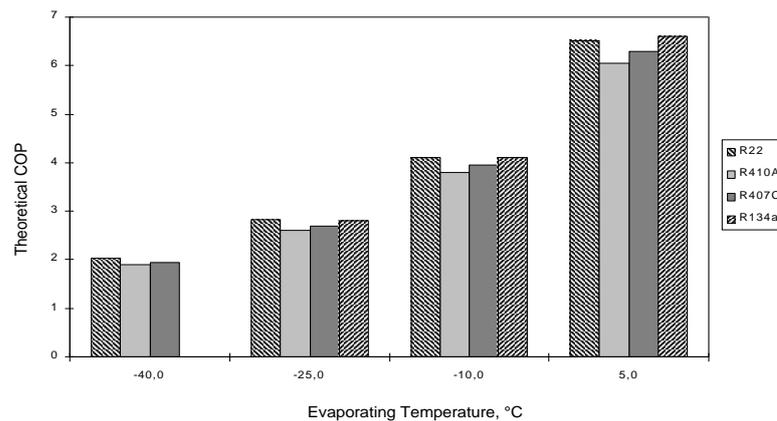
Fig. 1 Comparison of theoretical COP for refrigerants (Condensing temperature 40°C, suction superheat 20K, zero subcooling.)
