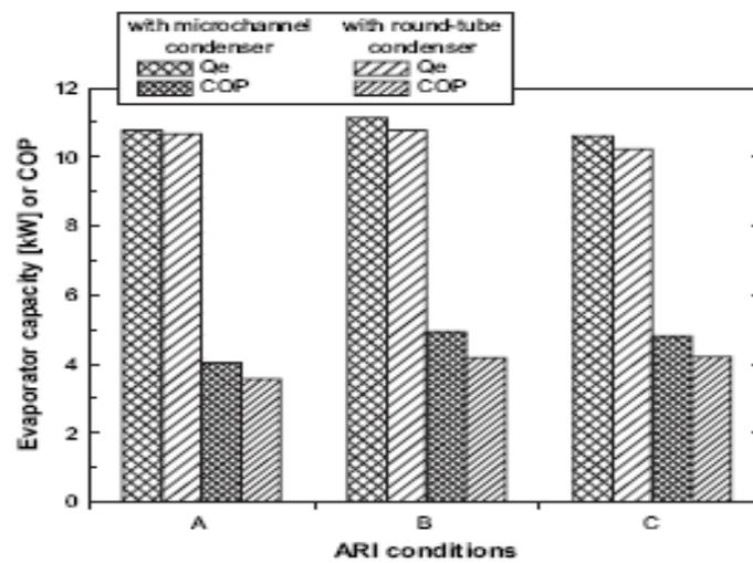
Fig. 6 Comparison of evaporator capacity and COP
