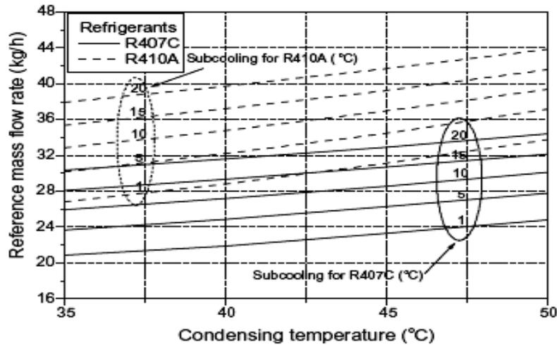
Fig. 7 Reference mass flow rates for R407C and R410A (Reference capillary tube: L =1500 mm and D =1.21 mm)
