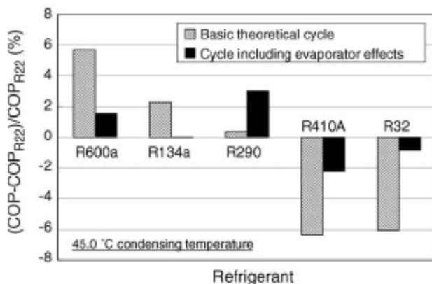
Fig. 9 (b) COPs compared to the COP of R22 for the basic cycle and for the cycle including evaporator effects for 45.0° C
