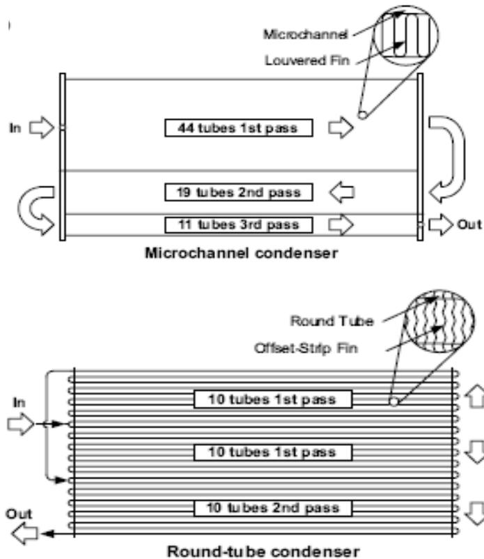
Fig. 4 Schematics of the unfolded microchannel and round-tube condensers
