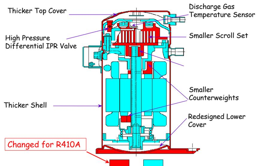
Fig. 3 ZP Scroll Compressor Showing Changes Made for R410A
