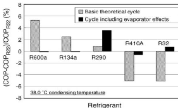
Fig. 9 (a) COPs compared to the COP of R22 for the basic cycle and for the cycle including evaporator effects for 38.0° C
