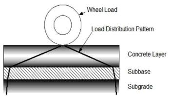
Fig 2. Load distribution of rigid pavement.
