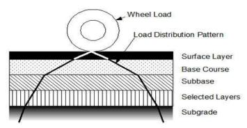
Fig 1. Load distribution of flexible pavement.
