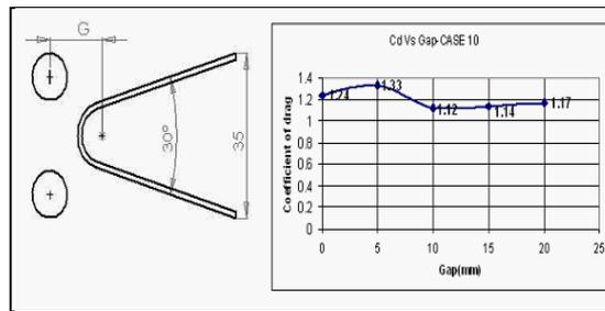
Fig 14: Configuration and  $C_d$  Vs Spacing gap for case 10
