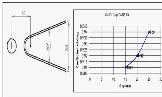
Fig 18: Configuration and  $C_d$  Vs Spacing gap for case 13.
