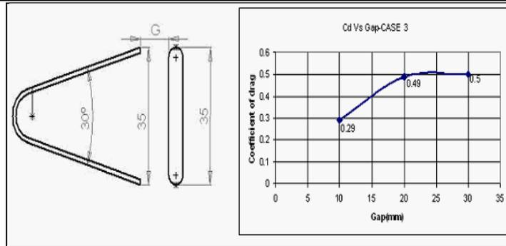
Fig 5 Coefficient of drag Vs Gap between the rounded edged disc and gutter
