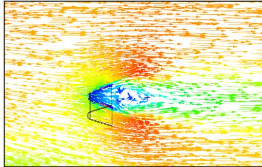
Fig 2: Flow pattern over the V-gutter
