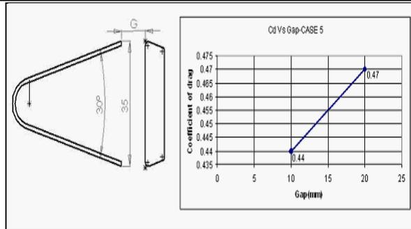
Fig 8: Configuration and Cd Vs Spacing gap for case 5
