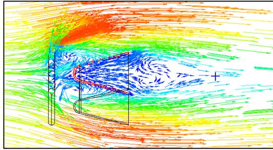
Fig 11: Flow pattern of the disc of 35mm width upstream of the gutter
