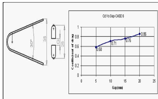
Fig 9: Configuration and  $C_d$  Vs hole size for case 6
