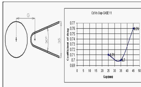
Fig 15: Configuration and  $C_d$  Vs Spacing gap for case 11
