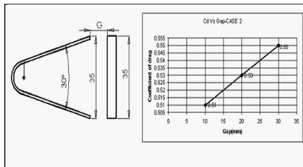
Fig 3: Coefficient of drag Vs Gap between the flat edged disc and gutter
