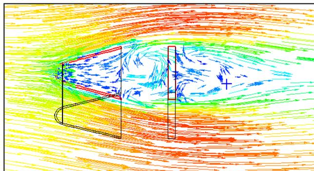
Fig 4: Flow pattern over the gutter with flat edged disc in tandem
