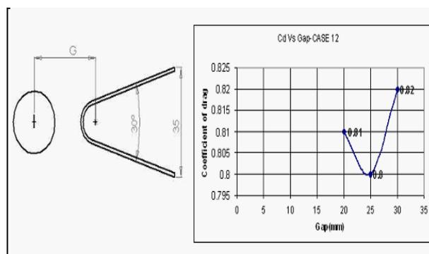
Fig 16: Configuration and  $C_d$  Vs Spacing gap for case 12
