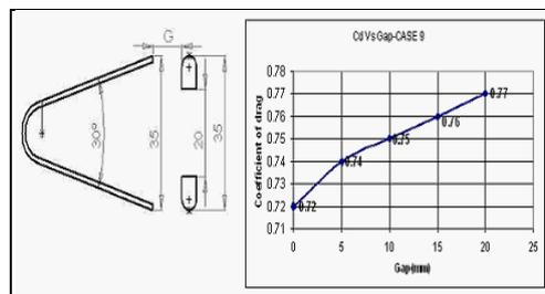
Fig 13: Configuration and  $C_d$  Vs Spacing gap for case 9
