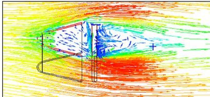
Fig 6: Flow pattern of rounded edged disc downstream of the gutter
