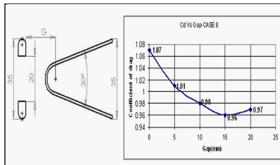
Fig 12: Configuration and  $C_d$  Vs Spacing gap for case 8
