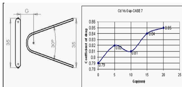
Fig 10: Configuration and  $C_d$  Vs Spacing gap for case 7
