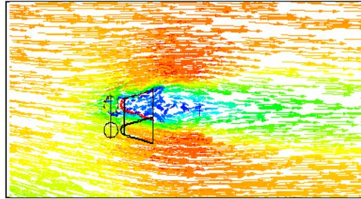
Fig 17: Flow pattern for 20mm circular ring upstream of the gutter
