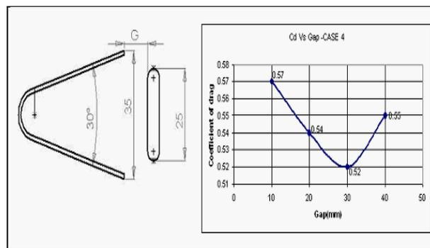
Fig 7: Configuration and  $C_d$  Vs Spacing gap for case 4
