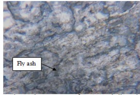
Fig. 5 Microstructure of Zn-22%Al alloy with 2% fly ash.
