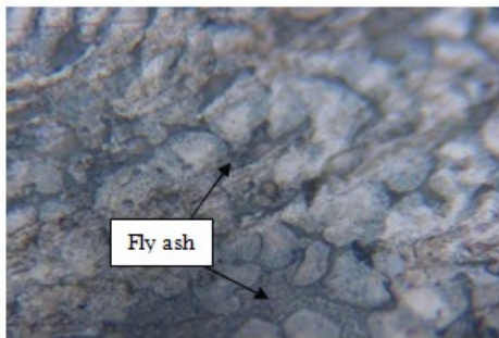
Fig. 6 Microstructure of Zn-22%Al alloy with 4% fly ash.
