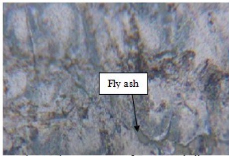
Fig. 4 Microstructure of Zn-22%Al alloy.
