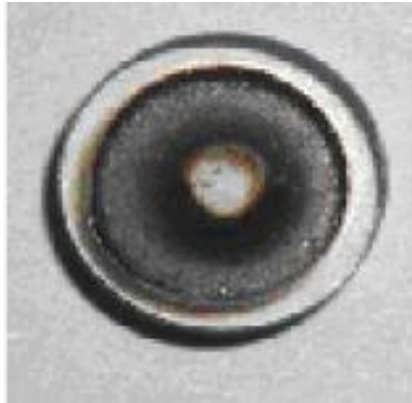
(b) Immediately after 100 pulses laser, Beam area is cleaned by the laser beam.
