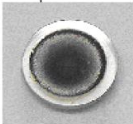
(a) After 20 hr operation with spark plug ignition, heavily polluted
