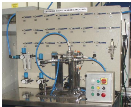
Figure 3–Experimental setup for levelling valve flow measurement.
