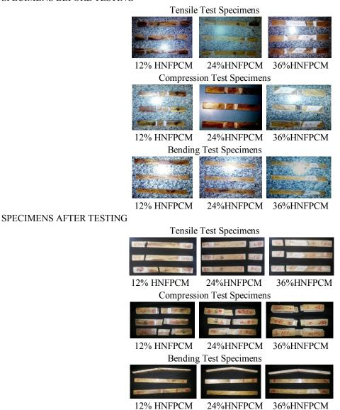
Fig 3.1: Fabricated Specimens Before and After Testing
