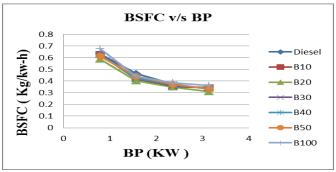
Fig 3: Brake specific fuel consumption v/s Brake power
