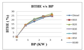
Fig 2: Brake thermal efficiency v/s Brake power
