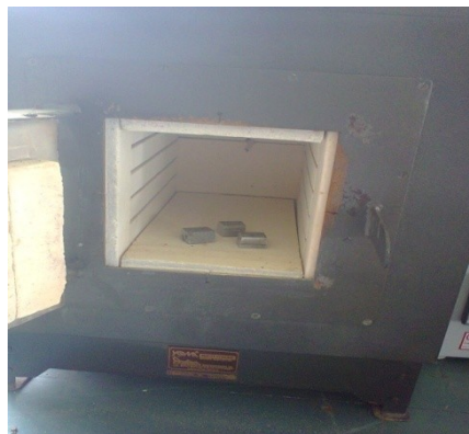
Fig 3.3 Muffle furnace containing workpieces for heat treatment
