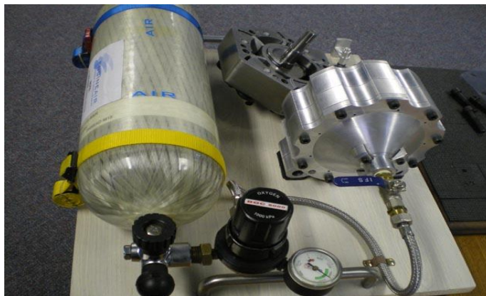
Fig2: Compressed Air Engine with modified tank
