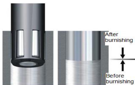
Fig. 3. Surface before and after roller burnishing [18]
