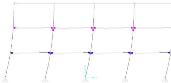
Fig8-c Plastic hinges in RC building propagates to the intermediate column
