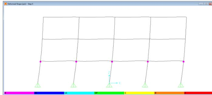
**Fig9-b Plastic hinges in RCS building propagate to the outer columns of the lower story**
