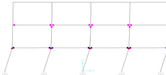
Fig8-d Plastic hinges in RC building propagates to the external columns
