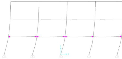
Fig8-a Plastic hinges in RC building starts at beams of lower floor
