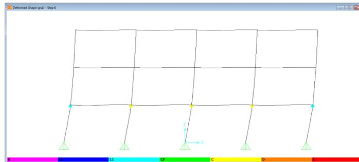
**Fig9-c plastic hinges in RCS building at failure**
