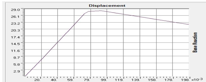
Fig. 4 displacement vs base shear for RCS structure
