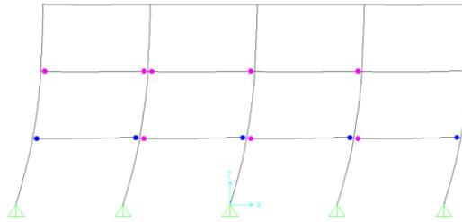
Fig8-b Plastic hinges in RC building propagates to the at beams upper story
