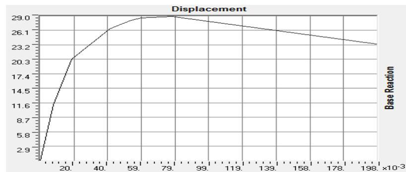
Fig. 5 displacement vs base shear for RC structure
