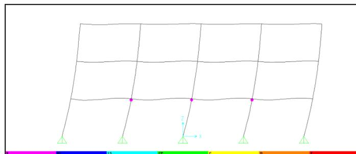
Fig9-a Plastic hinges in RCS building starts at intermediate columns of the lower story
