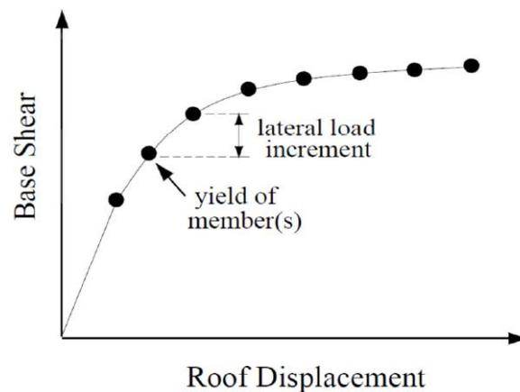
Fig.1 Expected Capacity Curve of the frame element
