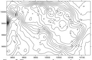
Figure 7: The contour map of test area based on photogrammetric methods
