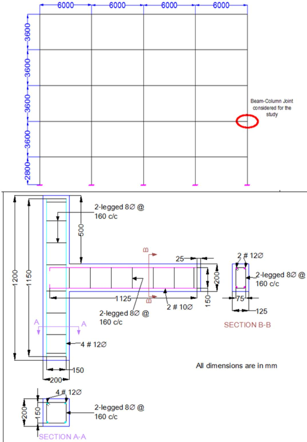
Fig. 1 General Arrangement of the Building Frame Considered for the Study
