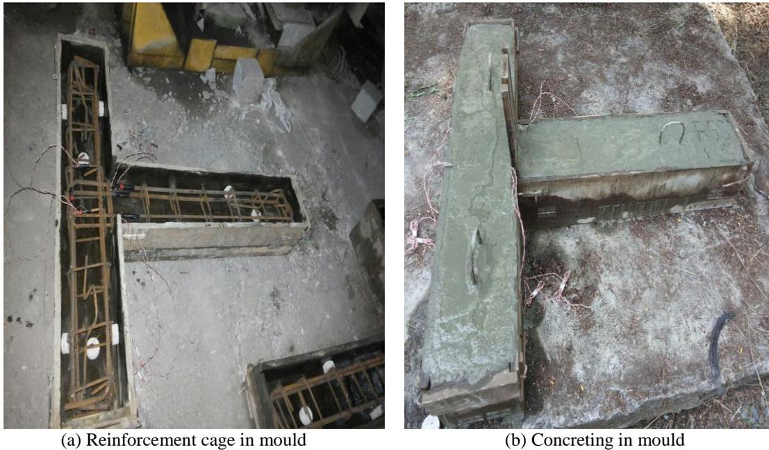
**Fig. 3 Preparation of Test Specimen**
