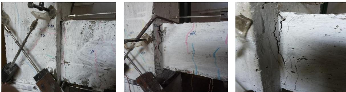
Fig. 5 Crack and Damage Pattern of Beam-Column Specimen
