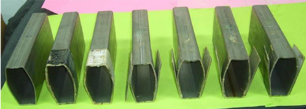
**Fig. 6 Failure modes of stainless steel section F120 x 40 x 3 using different FRPs**
