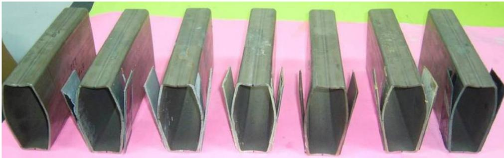
**Fig. 5 Failure modes of stainless steel section F120 x 40 x 3 using different adhesives.**
