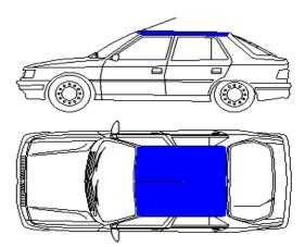
In order to avoid those problems, the usage of air conditioner is replaced by the phase change material. In this case, the air conditioner is taken out and top cover is filled with the phase change material. The Phase change material is filled in the aluminium pouch and sealed. These pouches are installed inside the car at the top cover. Thus Phase change material extracts the heat inside the car. The amount of heat extracted is depends on the mass of the phase change material.
