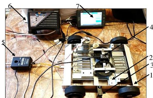
**Fig. 23** illustrates the experimental set up where: 1 – is body1; 2 – body2; 3 – accelerometers #1; 4 – accelerometer #2; 5 – load sell; 6 – new power supply & speed controller; 7 – LabQuest 2 unit.
