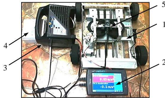
**Fig. 10** illustrates the equipment used in the forced vibration test, where: 1 is the shaker (body 2); 2 - LabQuest 2 unit, 3 – the power supply unit, 4 - motor speed controller: 5 - accelerometer # 2
