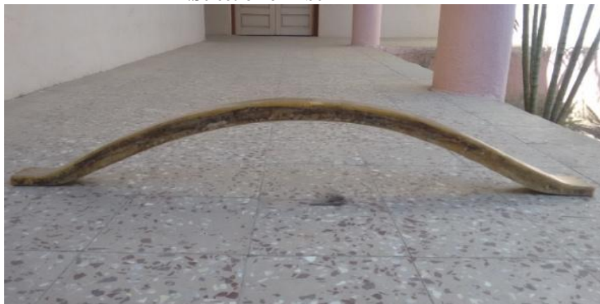
Fig. 1- Fabricated composite Leaf Spring
