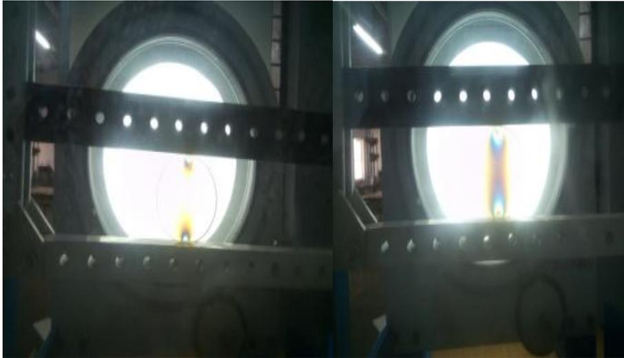
Fig. 3.1.Fringe patterns observed on disc due to loads 20N,40N,80N,100N
