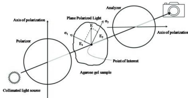
Fig2.2 Elements of Polariscope.
