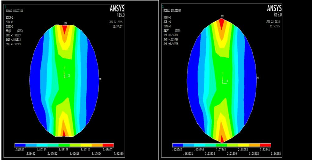
**Fig. 4.1 . Stress contours on circular disc obtained through ANSYS.**
