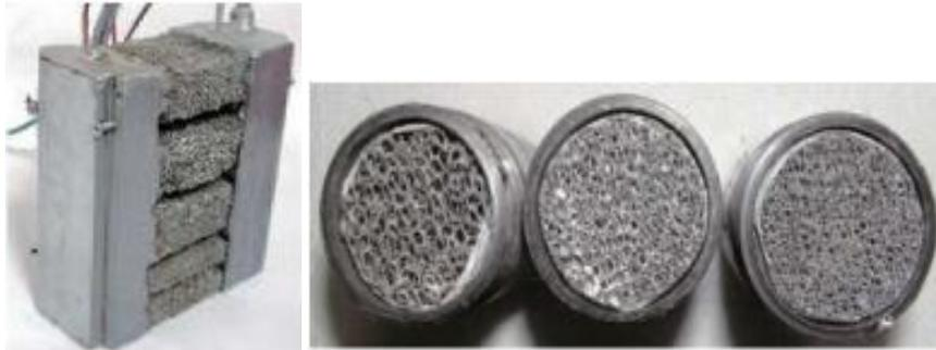
Schematic of prototype water heater made of open cell aluminum and heateropencell aluminum of 10, 20 and 30 PPI
