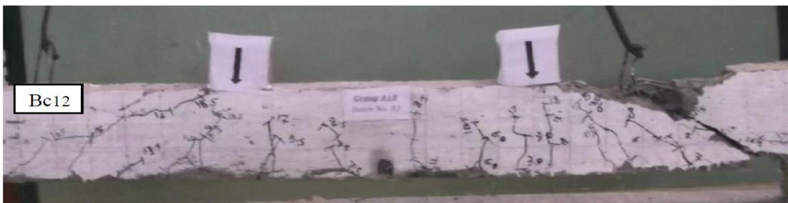
**Fig. (26):** Shape of failure of beam (Bc12)
