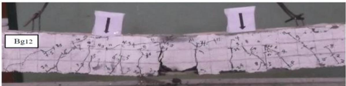
**Fig. (24):** Shape of failure of beam (Bg12)
