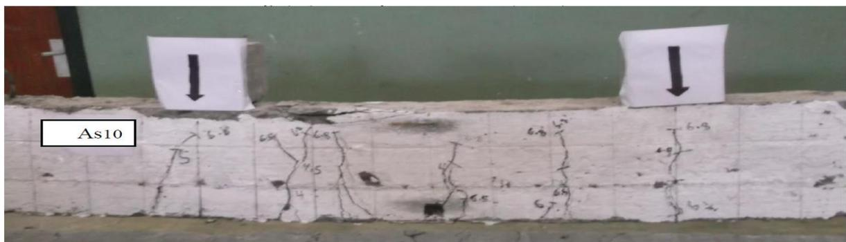
Fig. (22): Shape of failure of beam (As 10)
