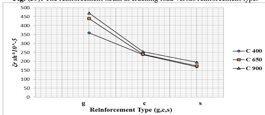
**Fig. (60):** The reinforcement strain at shear load ( $\xi_{rsh}$ ) versus reinforcement type.
