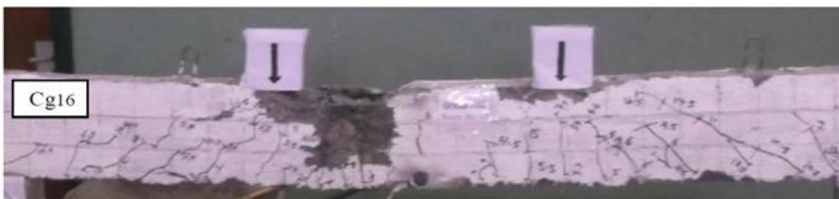
Fig. (30): Shape of failure of beam (Cg16)
