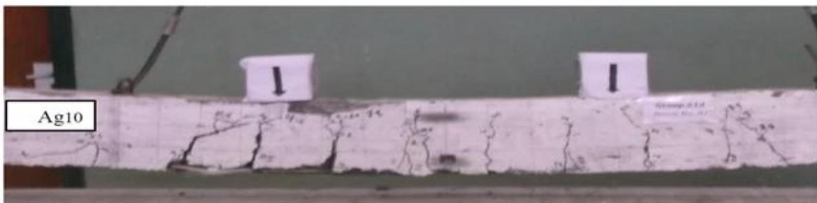
Fig. (18): Shape of failure of beam (Ag10)
