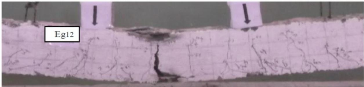
**Fig. (12):** Shape of failure of beam (Eg12)
