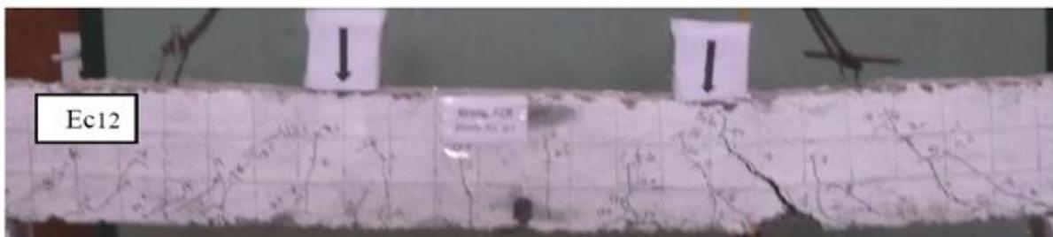
**Fig. (14):** Shape of failure of beam (Ec12)
