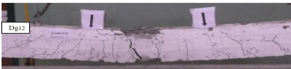
**Fig. (6):** Shape of failure of beam (Dg12)
