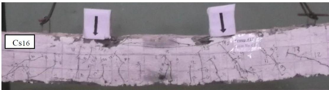
Fig. (34): Shape of failure of beam (Cs16)
